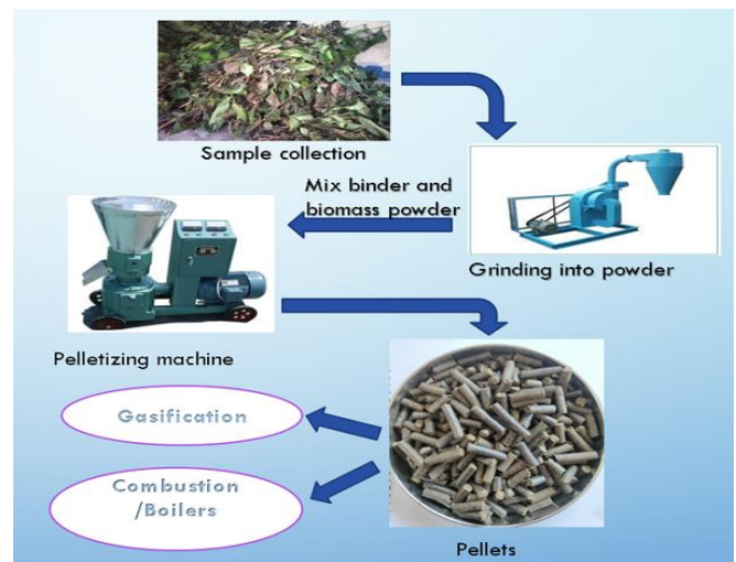
Figure 2. Schematic representation of production of tea biomass pellets (Source: Authors' own elaboration)
