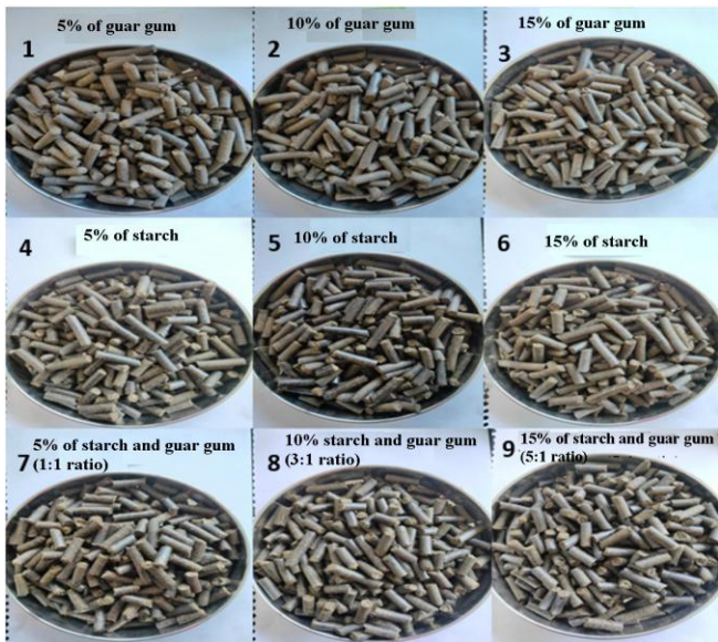
Figure 3. Biomass samples of different binder concentrations (Source: Authors' own elaboration)
