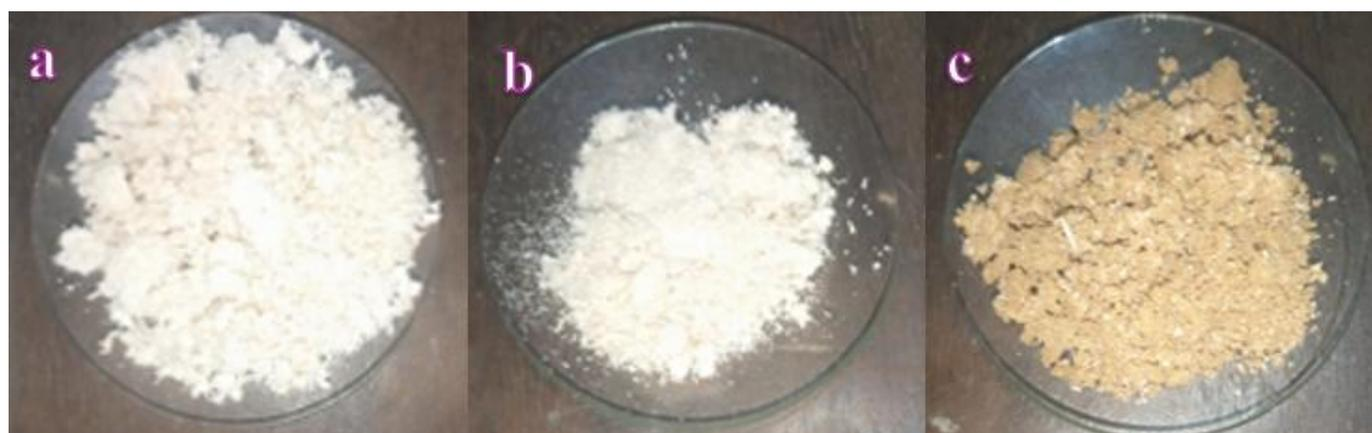
**Figure 4.** Bleached cellulose samples (a- beans peel, b- plantain peel, c- wooden wine cork) (Source: Field study)
