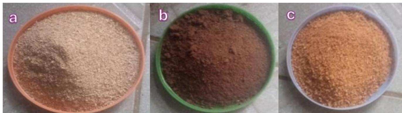
**Figure 2.** Pictures of plant waste materials after grinding (a- ground beans peel, b- ground plantain peel, c- ground wooden wine cork) (Source: Field study)
