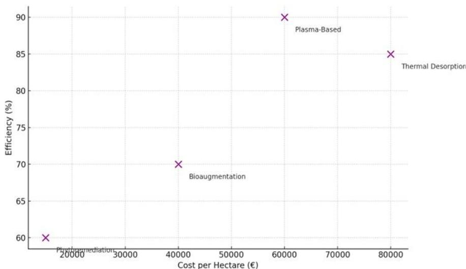
**Figure B1.** Cost vs. efficiency of PFAS remediation methods (derived from Goldenman et al., 2019 and Ross et al., 2018)
